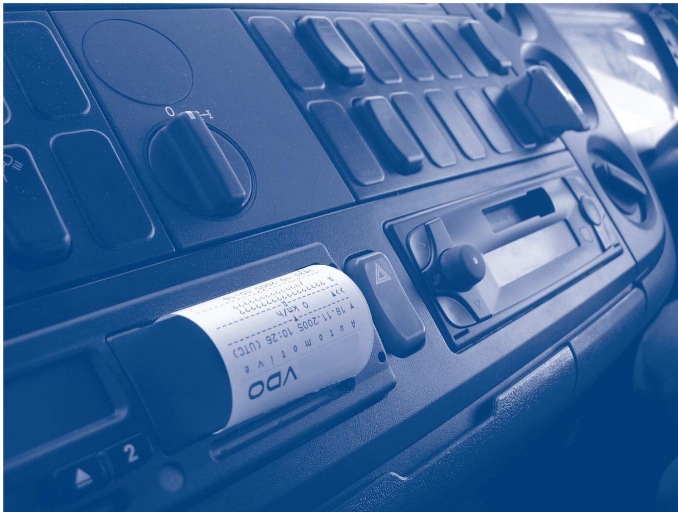
Digital tachographs work by storing digital data on the driver and vehicle in their own memory and separately on a driver's smart card. Transport undertakings must periodically download this data from the digital tachograph (known as the Vehicle Unit or VU) every 56 days and from driver cards every 28 days, and analyse the information to ensure that the rules have been complied with.
